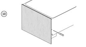
Insert a Phillips screwdriver into the hole above each side pin and rotate to adjust the panel alignment. There is a maximum travel distance of  $\pm$  1/16" (2mm).
