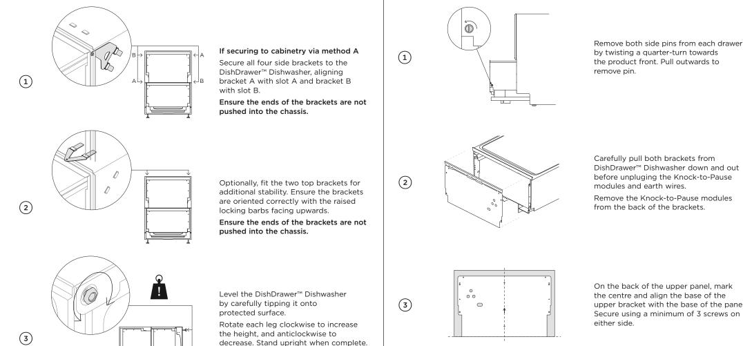
On the back of the upper panel, mark the centre and align the base of the upper bracket with the base of the panel. Secure using a minimum of 3 screws on
