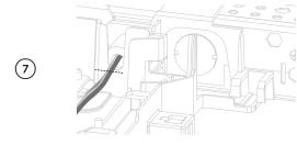
Carefully remove the cord from the product. Set toroid aside to for later use.
