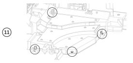
Lock clips back into place by pressing down on the cover firmly. Ensure all illustrated areas are engaged.
