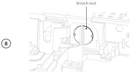
Fit a suitable cable clamp for the conduit through the metal knockout. Route wiring behind the tab and through the toroid removed earlier.
