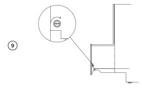
Re-insert both side pins to each drawer by pushing in and twisting a quarter-turn towards the rear of the product to secure panels into place.
