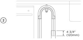
Pull both hoses through the support guide and rest in standpipe.
