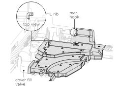
Position the cover fill valve into place before lowering the rest of the cover into position.
