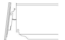
Carefully fit the panels onto the product. When refitting the lower panel, we recommend pushing back the drawer slides as shown on page 10 for access.
