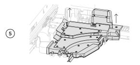
Lift the cover upwards until you are able to pull out towards you to remove.
