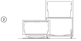
Lift the drawer off the runners and carefully set aside on a protected surface. Push runners back in.
