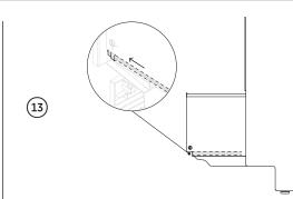
Ensure the hoses are not twisted before refitting the drawer to the runners and clipping into place via both locking tabs.
