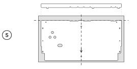
Snap the bracket tab to remove.
