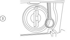
Pull the door release tab down from the ring. Use a screwdriver tip, pen or key to get a good grip.
