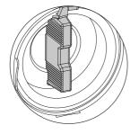
Replace the filter by turning clockwise until the turning handle stops in the vertical position, and cannot be turned further.
