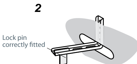
Fig. 18c Fitting the lock pin through the bracket
