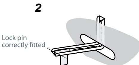
Fig. 6b Fitting the lock pin through the bracket
