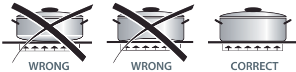
Fig. 52 Inefficient and efficient saucepan bottoms
