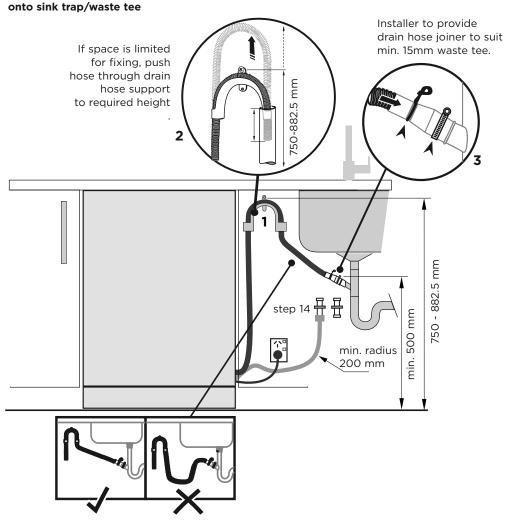
Ensure drain hose is routed straight to joiner. Remove *excess* drain hose material if necessary. **Do not shorten the inlet hose**.
