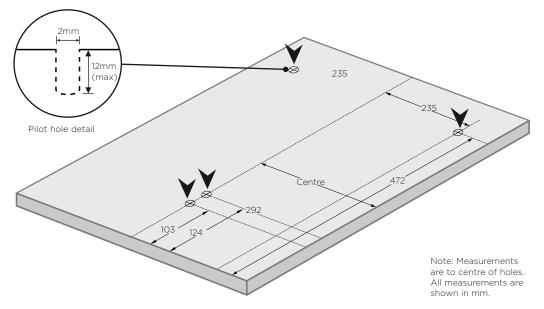
**2B** If the overhang of your panel is between **54mm and 74mm** use the below guide to mark out the locations for your fixings.
