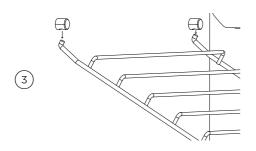
Swing the bottom of the side rack up towards the center of the oven until it is almost horizontal. Slide the prongs at the top out of the mounting slots.
