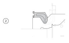
Open the hinge locks fully on both sides
