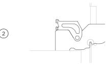
Open the door completely and ensure both hinges are secured by the correct notches.
