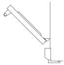
Holding the door on both sides, lift door back up to  $45^{\circ}$  and carefully pull the door out and away from the hinges.
