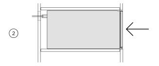
Push the warming drawer back into the cabinetry, and align the front panel with the cabinetry as desired.
