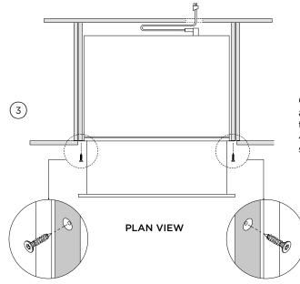
Open the drawer and secure the attachment flanges of the drawer to the side edges of cabinetry with 4x25 T20 star head countersunk screws.
