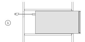
Connect the power plug into the power outlet.
