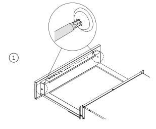
Open the drawer fully, and slightly loosen the screws.
