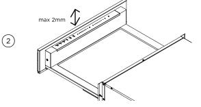
Adjust to the required height and then re-tighten the screws. The height is adjustable within 2mm.
