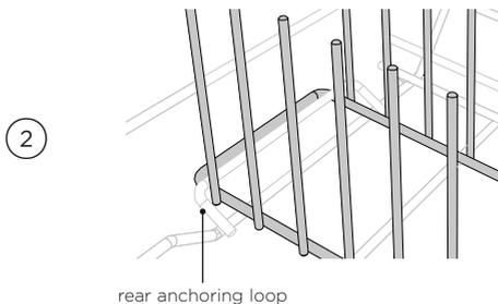
Lower the fixed tine rack into place and push in to hook under the rear anchoring loop.
