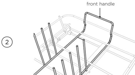
Using the handle at the front of the fixed tine rack, pull forward ensuring the rear anchoring loop is cleared before lifting out.
