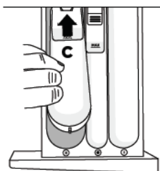
Replacing the liquid detergent compartment
