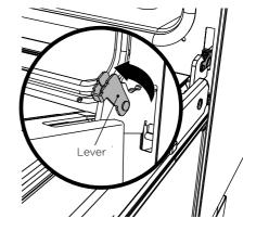
2 Open the levers fully on both sides.
