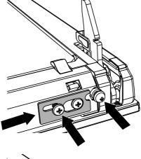
Se-tighten the screws so that the latches and the lower trim are firmly secured.
