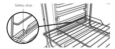
3 Tilt the front up slightly to help the safety stops clear the side rack wires.
