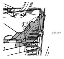
② Insert the hinge tongues into the slots, making sure that the notches on both sides drop into place as shown.
