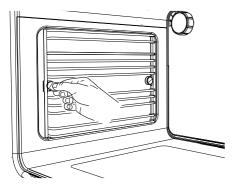
② Use a small coin or a flat-head screwdriver to loosen and remove the fixing screws.
