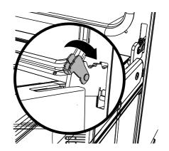
④ Fully close the levers on the left and right hinges, as shown, then close the door.
