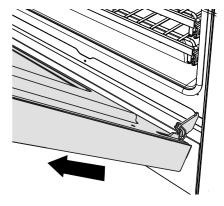
4 Disengage the hinges and remove the door. Place on a protected surface.
