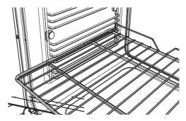
2 Position the shelf: it should rest on the side rack wires, as shown.
