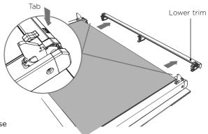
③ Press down on the tabs to release the lower trim and remove it.
