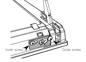
2 Slide the latches inwards so that the lower trim can be removed.
