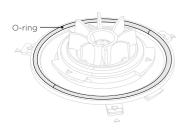
Before refitting the filter plate, ensure the O-ring is correctly positioned within the tub as shown. If the O-ring is incorrectly fitted before running a cycle, product damage may occur.
