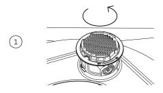
Twist the filter anti-clockwise until the arrow in the tub points to  $\widehat{\ }$  on the filter. Lift to remove.
