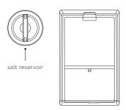
The salt reservoir is located on the inside of the drawer next to the detergent dispenser. It holds up to approximately 0.88lb (400g) of salt (actual capacity will vary depending on brand and grain size of salt used).
