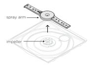
With racking removed, lift the spray arm off the impeller, pulling up from the centre. Shake to dislodge any loose particles, rinse under running water and wipe with a damp cloth. Ensure the magnet is clean and clear and that water can flow through all holes.
