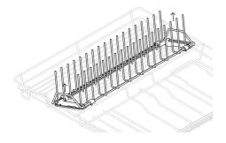
Grip the front and back handles and pull up to unclip.
