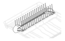
Slide the tines backward or forward by pushing or pulling the front handle.
