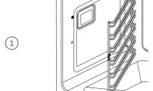
Slide the rear prongs of the side rack back into the holes, ensuring the rack is firmly pushed up against the side wall of the oven.
