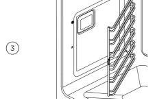
Slide the side rack forward until the rear prongs are clear of the holes.
