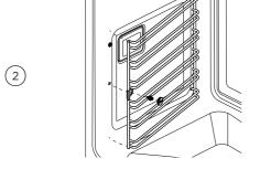
Fit the side rack front tab over the fixing screw.
