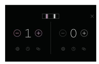
2. Press ⊝ or ⊕ to adjust the fan speed. There are 5 speeds plus BOOST. Press and hold ⊝ or ⊕ to jump to 0 or BOOST, respectively.
