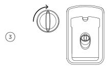
Refit the cap, turning clockwise until secure.
