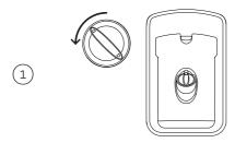
Turn the cap anticlockwise and remove.
