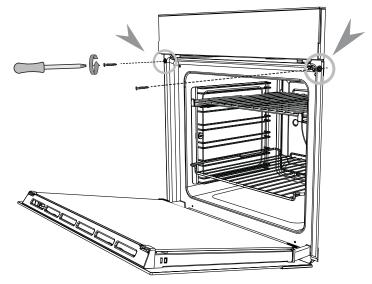
Make sure the oven is level and securely fitted to the cabinetry.
