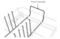
Using the handle at the front of the fixed tine rack, pull forward ensuring the rear anchoring loop is cleared before lifting out.
