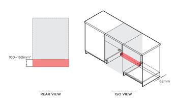
Service outlet at rear extends both sides, hoses and cords can be routed to either or both sides. \*Depending on adjustment of levelling feet.
