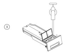
To clean the dispenser drawer, fill the compartments with warm water and shake lightly to clear residue. Drain all water from the compartments before re-fitting the dispenser drawer to the washer.
