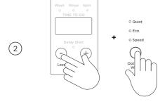
Press MORE  $\pm$ , LESS  $\pm$  and OPTIMISE WASH buttons together for three seconds, dEF will appear on the screen and the washer will beep.
