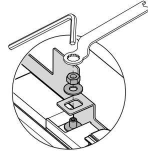
Loosely screw the M8 washer and nut to the stud using the hex key and spanner.
