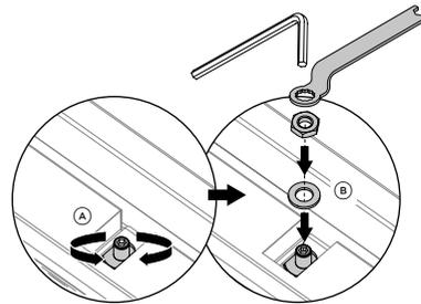
To adjust the height of the panel, turn the stud clockwise to raise or counter-clockwise to lower the door panel.
