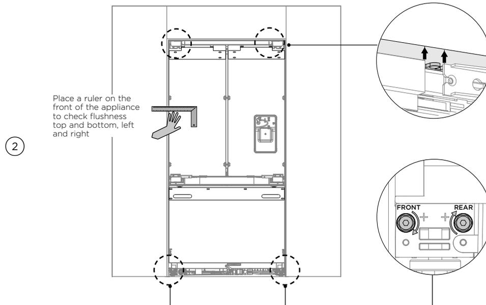
Place a ruler on the front of the appliance to check flushness top and bottom, left and right
