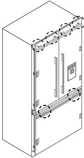
Open the door and loosen the M5x10 cross-head screws (do not remove) at the sides of the doors
