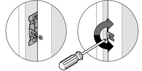
Slide the forks of the side brackets onto the screws of the door.
