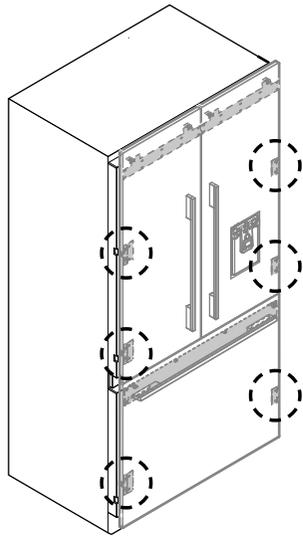
Slide the forks of the side brackets onto the screws of the door.
