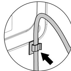
Secure the excess power cord length onto the clip. Be careful when pushing the appliance into position, to avoid roll over or damage to the power cord and/or water tubing.
