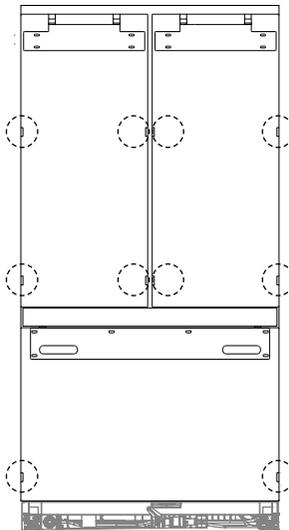
Loosely screw (1-2 turns) M5x10 cross-head screws into doors.
