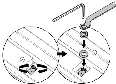
To adjust the height of the panel, turn the stud clockwise to raise or counter-clockwise to lower the door panel.
