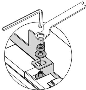
Loosely screw the M8 washer and nut to the stud using the hex key and spanner.
