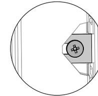
Secure side bracket forks by tightening side screws. Repeat for all door panels.
