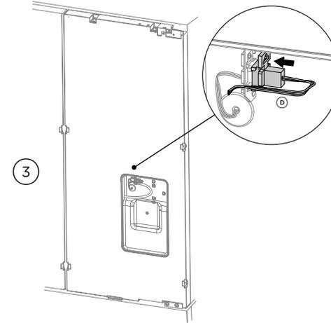
Connect the display harness onto the appliance door by inserting firmly until you feel it clip securely.
