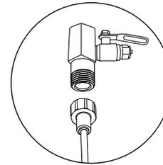
Connect the water tap adaptor to a water tap. Flush water through the hose prior to connection to the appliance to remove any debris in the hose.
