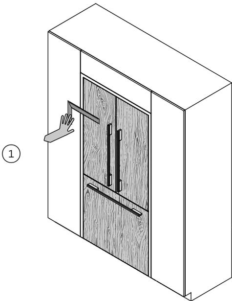
Push the appliance into the cavity until the door panels are flush with adjacent cabinetry surface.
