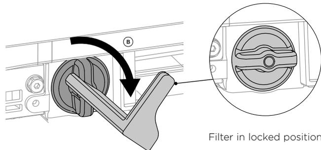
Align the filter removal tool over the filter handle and turn 90° clockwise to tighten. Remove filter removal tool and close the freezer drawer.
