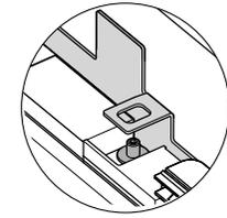
Open the door and loosen the M5x10 cross-head screws (do not remove) at the sides of the doors
