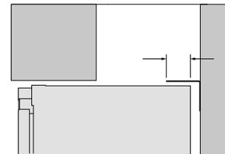
When rolling the appliance into the cabinetry, ensure the anti-tip bracket overlaps the back edge of the appliance.
