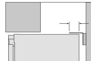
If minimum 7 1/16" (180mm) overlap cannot be achieved, install a solid spacer to the wall stud behind the bracket.
