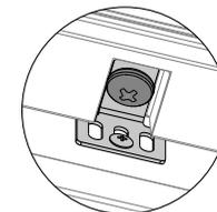
Loosen the M8x16 crosshead screw so that locking bracket can slide freely back to front. Slide the locking bracket out until it touches the back of the door panel. Fully tighten the screw.
