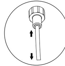
Connect the free end of the plastic tubing fully into a water tap adaptor. Pull gently to ensure it is locked in.
