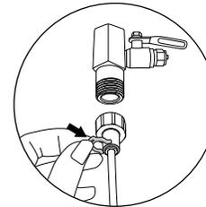
Secure the connection with a locking key inserted between the water tap adaptor and locking collet.
