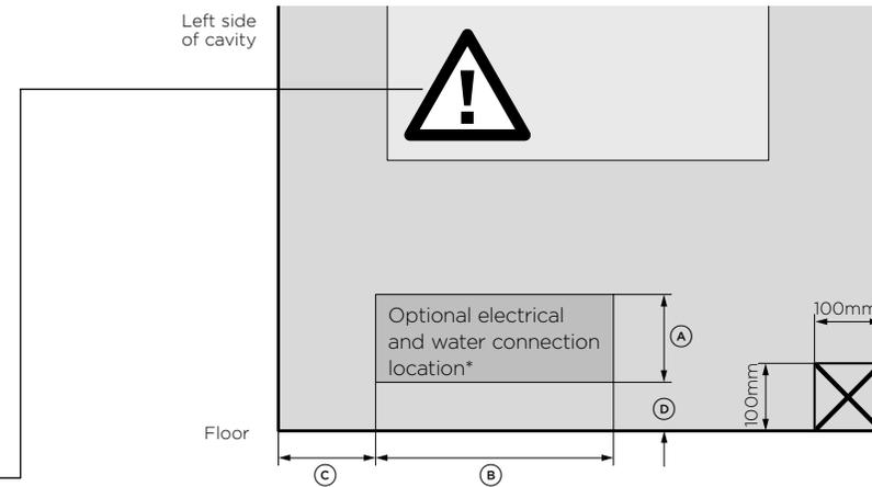
Electrical and water connections must be within this space if located behind the appliance and must not protrude from the back wall.
