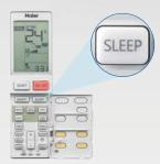
In cooling operation, temperature is set to be  $1^{\circ}\text{C}$  up in the 2nd hour, then maintains 6 hours before the unit turns off.
