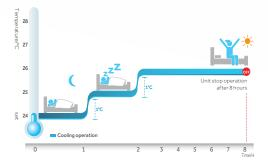
When using Sleep Mode to heat, the temperature drops 2°C per hour for two hours, maintains that temperature for three hours and increasing by 1°C for the remaining three hours, then deactivates.
