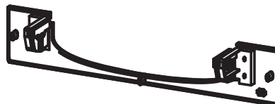
Toekick mounting bracket (1) (A custom toekick panel of any material with thickness 9 - 19 mm can be screwed to the plastic toekick mounting bracket)
