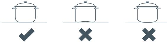
Fig. 16b Efficient and inefficient saucepan bottoms
