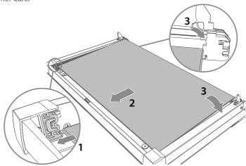
1 Take either one of the middle panes (B or C) and hold it firmly. Insert it in the lowest pair of grooves (1), push it slightly towards yourself (2) and gently lower into place (3).
