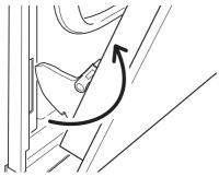
**5a** Lift the door and disengage the hinges.
