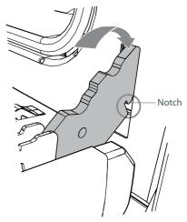
Insert the hinge tongues into the slots, making sure that the notches on both sides drop into place as shown.
