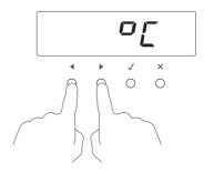
Press and hold the scroll ◆ ▶ buttons together for 3 seconds to enter the user preference menu.
