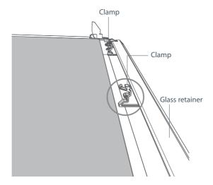
4 Position the glass retainer, as shown. It should sit on the bottom edge of the outer glass (A). Check that the clamps of the glass retainer are not deformed or damaged.
