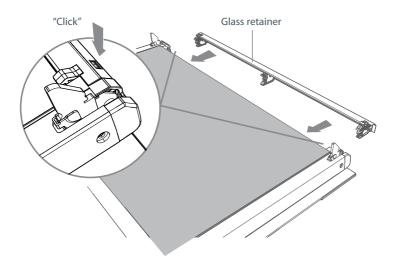
5 Gently push the glass retainer back into place. You should be able to hear the tabs on both sides click as they lock the glass retainer in.
