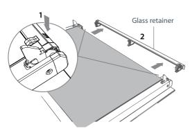
1 Press down on both tabs (1) to release the glass retainer (2).
