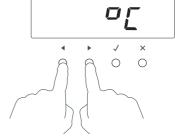
2 Press and hold the scroll ◀ ▶ buttons together for 3 seconds to enter the user preference menu.
