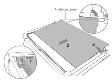
Take the inner pane (D), holding it with the angle-cut corner orientated as shown. Insert it in the uppermost pair of grooves (1), push it slightly towards yourself (2) and gently lower into place (3).
