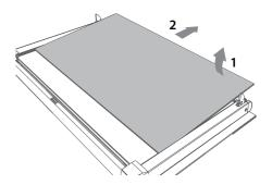
2 Lift the inner pane (D) slightly (1), then gently slide out (2).
