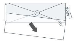
4 Carefully lift the glass cover out of the retaining bracket in the back and pull out the faulty bulb.
