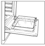
Fig. 41a Removing and replacing the oven door glass - OR60 models
