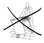
Fig. 18 Incorrectly lifting the cooker
