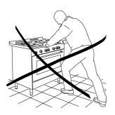
Fig. 17 Incorrectly moving the cooker
