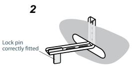
Fig. 20c Fitting the lock pin through the bracket
