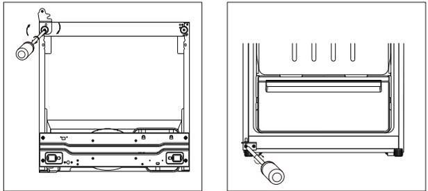
9. Make the middle hinge reverse the direction 180°, then transfer it to the left property position. Make the middle hinge pin in the upper hole of the lower door, then tight the bolts.
