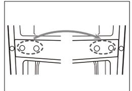
6. Unscrew bottom hinge. Then remove the adjustable feet from both side.
