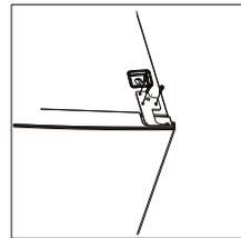
Unplug the temperature sensor from inside the top hinge cover and put the sensor back into the unit as shown below. Remove the door carefully and safely place to protect it from damage.
