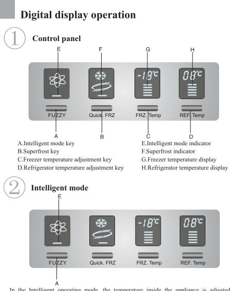
In the Intelligent operating mode, the temperature inside the appliance is adjusted automatically according to variations of the ambient temperature. Press key A once, upon which indicator E lights up and Intelligent mode is entered. Press key A once again, upon which indicator E goes off and Intelligent mode is cancelled.
