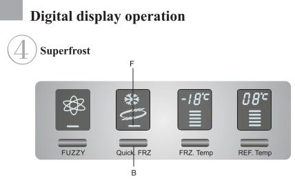
It has been scientifically proven that a Superfrost type device is necessary to freeze foods quickly and thoroughly. Press key B, upon which indicator F lights up and the Superfrost action is turned on. Press the key again to turn off the Superfrost action, upon which indicator F goes off. (In Intelligent mode, it is not necessary to turn on Superfrost.)
