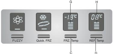
Refrigerator temperature adjustment: Press key D, upon which indicator H starts blinking. Each time key D is pressed, the temperature setting is increased by one of level from 1 to 5 (3 °C). If you keep pressing key D, the cycle starts over again from level 1 (7°C). Freezer temperature adjustment: Press key C, upon which indicator G starts blinking. Each
