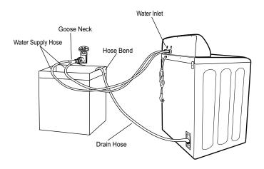
4. Plug the wash er into a regular 220-240 Volt/50 Hz, IOAmp outlet.
